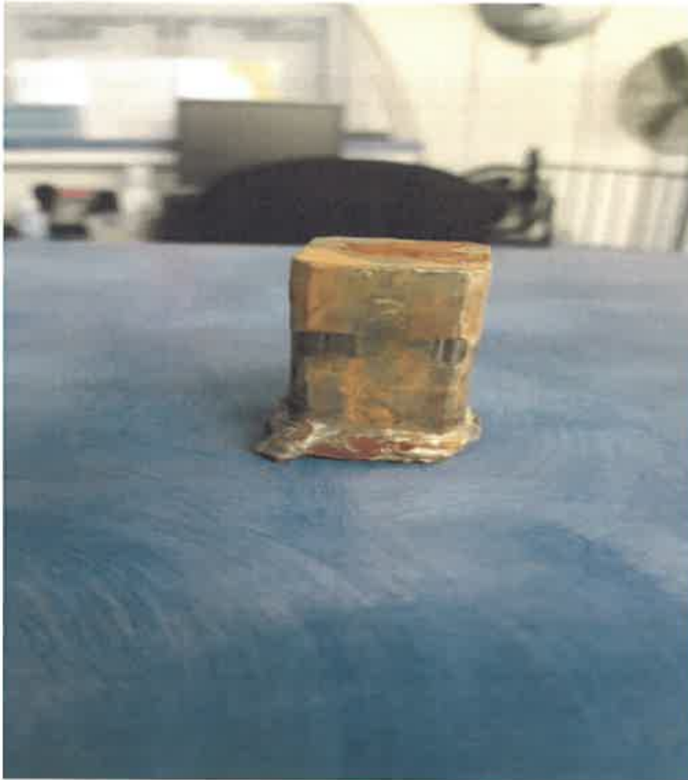
DETACHED SHAFT STEM WHICH TURNS THE VALVE
