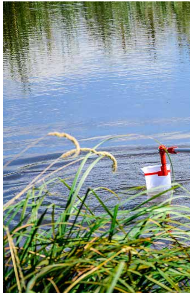
Sampling collection using a extended bucket to prevent contamination.
