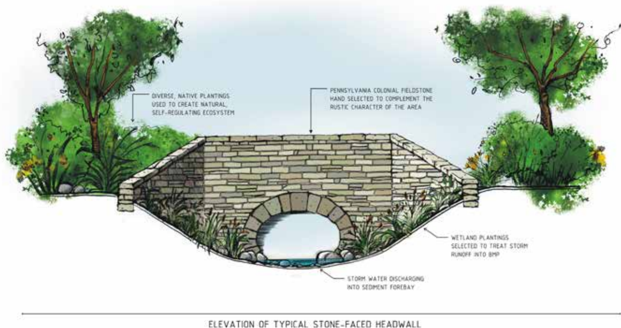
Rendering for a typical stone-faced headwall used throughout the Staten Island Bluebelt in New York City, NY
