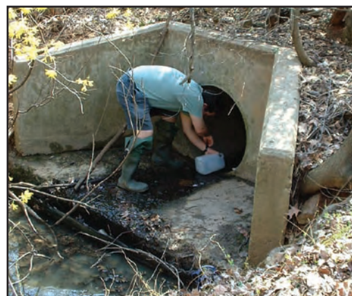
Figure 30: Measuring flow (as volume per time)
