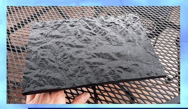
To Scale Up The Model Had To Be Broken into Pieces to Fit Printer
