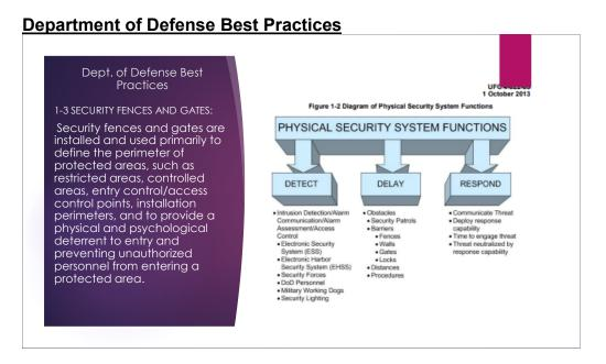
Security fences and gates are installed and used primarily to define the perimeter of protected areas, such as restricted areas, controlled areas, entry control/access control points, and installation perimeters, and to provide a physical and psychological deterrent to entry and to prevent unauthorized personnel from entering a protected area.
