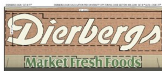
1 DIERBERGS SIGN: 107.8 FT 2 1 DIERBERGS SIGN CALCULATION PER UNIVERSITY CITY ZONING CODE SECTION 406.0200: 107.8 FT 2 x 12.0 FT = 1294.56 FT 2 1 MARKET FRESH FOODS SIGN: 147.4 FT 2 1 MARKET FRESH FOODS SIGN CALCULATION PER UNIVERSITY CITY ZONING CODE SECTION 406.0200: 147.4 FT 2 x 12.0 FT = 1768.8 FT 2 1 DIERBERGS - NORTH DATE: 07/17/17
