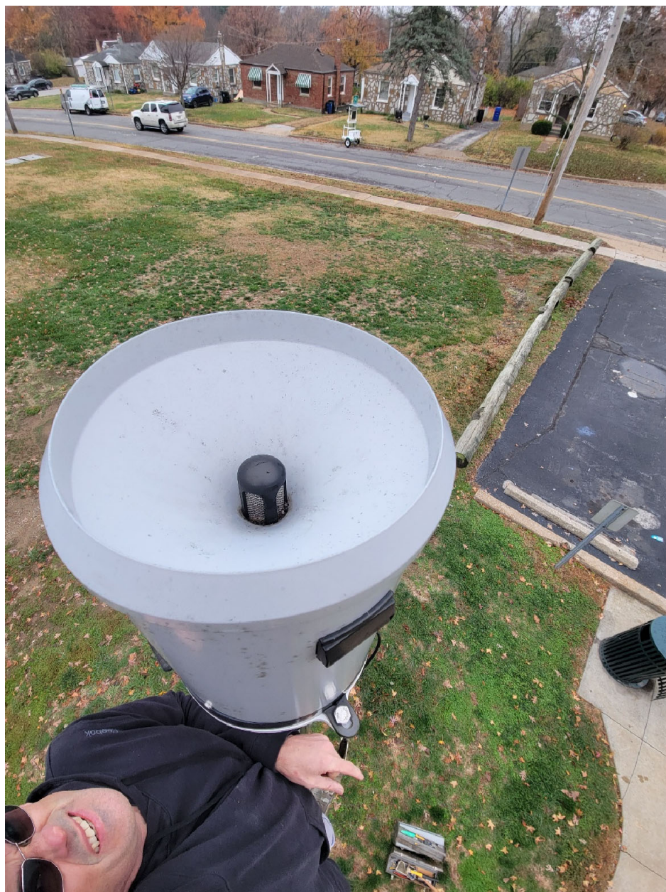
Figure 6 – Gage tipping bucket catchment. No obstructions.
