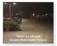
In addition to energy savings, the true success is indicated in the appearance and light distribution of the new fixtures. Because of the natural color temperature of the light output, CMH light provides a much truer color representation than HPS. The pictures above show the improvement of the distribution of light and the clarity of colors with the new lights.
